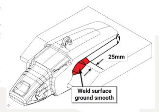
Welds shall be ground such that the surface of the weld becomes a smooth surface free of any roughness or ripples associated with fresh welds. The toes of the weld shall transition to the lip and Talon Adaptor smoothly, such that the transition exhibits a minimum of a 3 mm / 1/8" radius.
