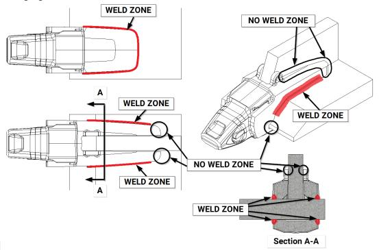
Preheat and fix the Adaptors in place with one 25mm / 1" tack weld at the root of the weld prep on either side of the top leg in the weld zone. Begin welding on the bottom of the Adaptor and complete first welding sequence in steps as per the Talon standard Adaptors as follows:
