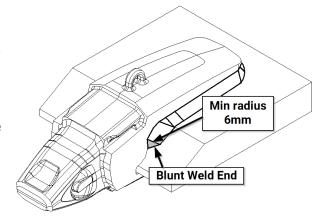
The surface of the fillet welds shall also be ground smooth for a minimum of 25mm / 1" back from the ends of the welds. For welds on the top surface of the lip that transition ramp face of the lip to the top surface of the lip. The surface of the weld shall be ground smooth from the weld end through to a minimum set back of 25mm / 1" back from the ramp face to top surface transition. (See figure adjacent)
