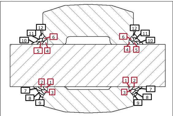
Recommended Talon Adaptor alternating weld sequence:
