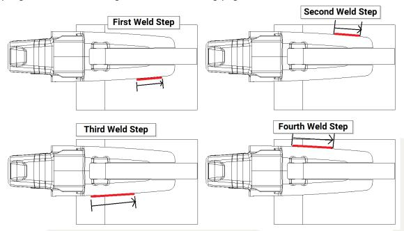
Continue to alternate welding between the top and bottom of the Talon straddle leg Adaptor and alternate between Adaptors as described on page 4 until the full weld size is achieved. The final fillet weld size should be such that the weld leg is approximately 5mm above the edge of the cast weld prep in the Adaptor. The weld should not undercut the weld prep. The fillet should be equal legged. The weld should form a profile as follows:
