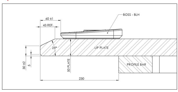
Lip profile must be relatively smooth and free of debris, such as weld spatter, metal deformation, cutting dags or other irregularities
