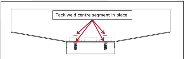
Place Half Arrow corner segments on the lip and tack in place with a 25mm / 1" tack weld on the bottom rear edge and two 25mm / 1" tack welds in the top weld gap.
