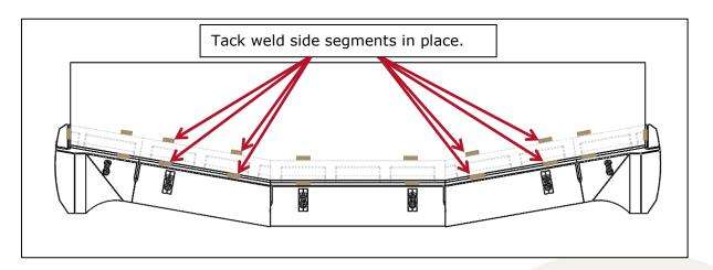
Complete a full root run and one capping pass along in the top weld gap followed by a full root run and one capping pass along the bottom edge of the Half Arrow. Following this proceed to fill out the welds as suits your welding equipment.
